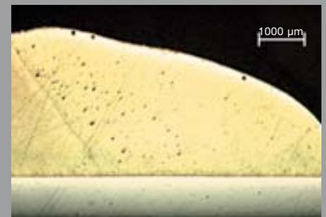
CMT joint between steel and aluminium. Welded on the aluminium side; brazed on the steel side.
