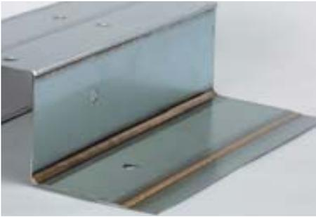
*CMT-brazed joint between hot-dip and electrolytically galvanized sheet. Sheet thickness 1.0 mm, filler metal CuSi3.*
