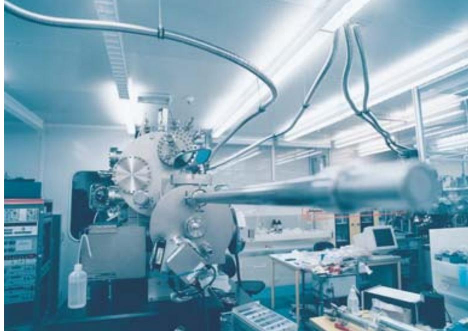
Epitaxy plant in the cleanroom of the Institute of Semiconductor and Solid-State Physics at the Johannes Kepler University, Linz. This is used for depositing semiconductor heterostructures with atomic scale precision.
